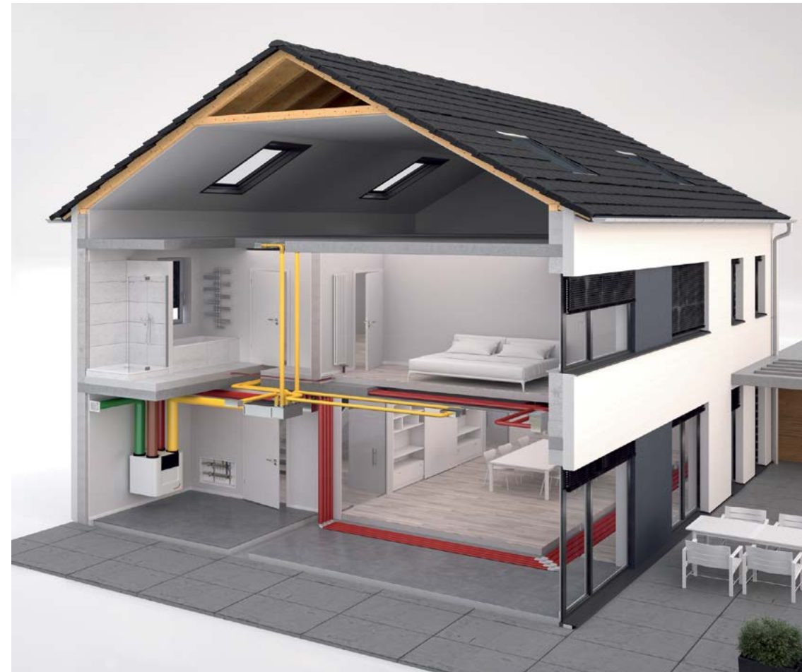
The yellow ducting shows where the moist, stale air is being extracted from wet areas; the red ducting illustrates the fresh, filtered air being delivered to bedroom and living areas. The heat exchanger uses the energy from the exhaust air (brown) to heat or cool the incoming outside air (green).
